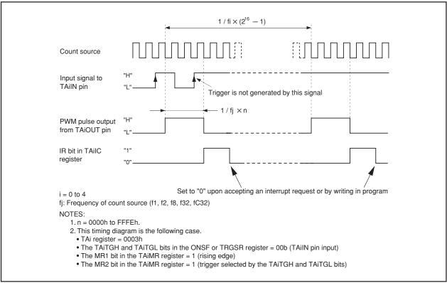
Figure 12.13 Example of 16-bit Pulse Width Modulator Operation
